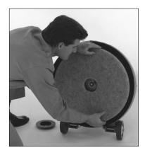
We recommend using NSS Ultra-High Speed Pads with the Charger 1500. These pads are specifically designed for use with all NSS ultra-high speed machines. They are a mixture of natural (75 percent) and synthetic fibers. The natural fibers give NSS pads the strength to keep their shape during prolonged use at ultra-high speeds. Polyester is added for the flexibility necessary to conform to the floor's contours.
